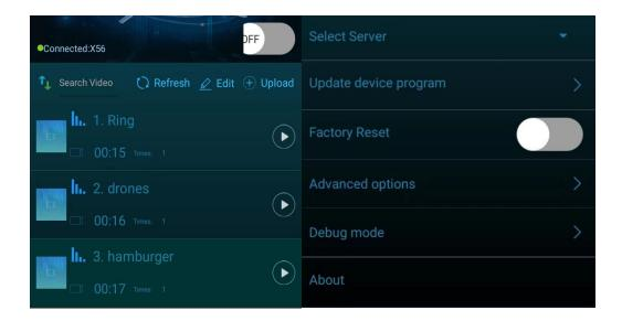
When you forget the WIFI password of the device: Press and hold the "NET" button on the back of the device for more than 10 seconds until the various colors of the indicator lights flash, the master machine returns to red, and the slave machine returns to yellow-green, indicating that the factory settings have been restored.
