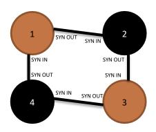
(2) The SYN OUT of device 1 is connected to the SYN IN of device 2, the SYN OUT of device 2 is connected to the SYN IN of device 3, the SYN OUT of device 3 is connected to the SYN IN of device 4, and then the SYN OUT of device 4 is connected to the SYN IN of device 1. SYN IN. As shown below:
